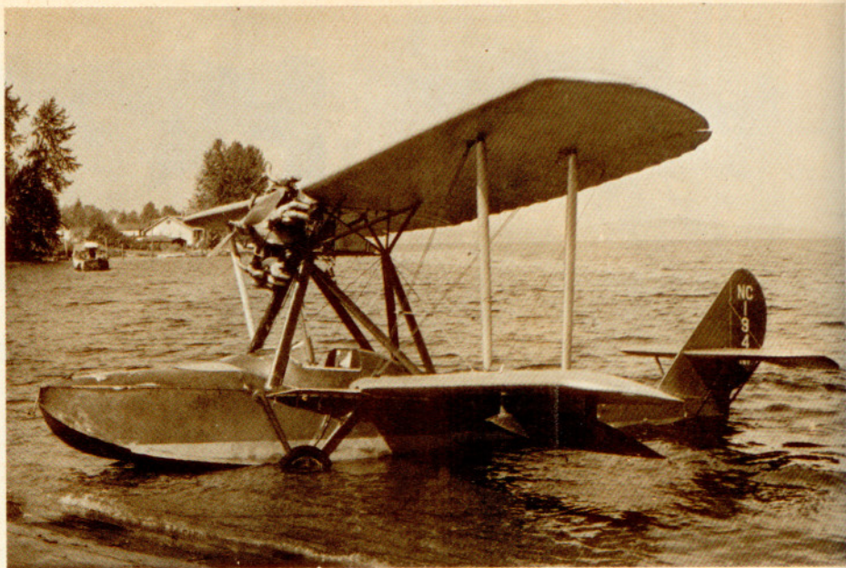
Overall design of the S-56 originated in World War I. Note the scalloped effect produced by the wire trailing edges of the wings
